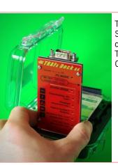
The dock in Shuttle Mode connected to a TRAFx Vehicle Counter
