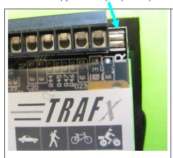
Create an electrical short by bridging between the two contact points in the white box above "**R**" with a ball point pen. This will reset the external LCD tally display to zero. (It does not affect the data stored in the counter's memory.)
