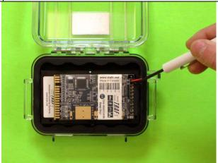
Step 1: Open the TRAFx Vehicle/OHV/Mountain Bike Counter field case; loosen screws and disconnect battery holder wires (red and black); remove circuitboard (it is attached with Velcro).
