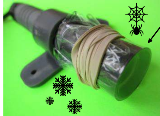
Overlap two pieces for 1/8 inch density
