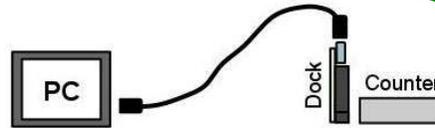
As a vehicle passes within the detection zone, or as you move a ferrous metal object (pliers, hammer, stapler – but not a magnet or magnetic screwdriver) near the counter (approx. 10cm / 6in.), this should trigger a count which appears on the PC's screen. Try it. Ferrous metal objects (i.e., metals with iron content) distort the earth's magnetic field as they move through it, and this triggers a count. Pure aluminum (non-alloy aluminum) will not be detected.
